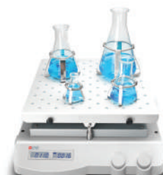
SK-R330-Pro LCD Digital Rocking Shaker Rocking motion angle 9° 10kg and speed range 10-70rpm
