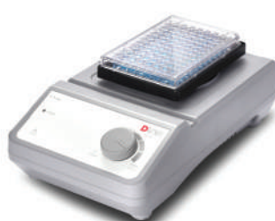
Microplate Mixer Motion type: Orbital Speed range Single microplate: 0-1500rpm|Double microplate: 0-1000rpm
